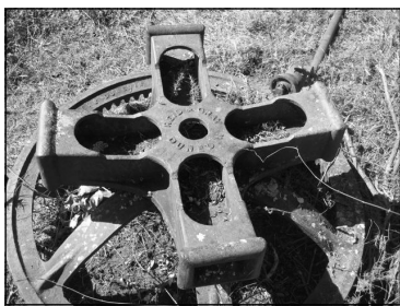
A picture of the whim. The four sockets are on the top. The toothed gear wheel can be seen underneath and the drive-shaft is at the top right.
