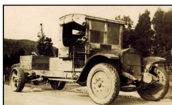
The early truck with solid rubber tyres at the back and inflated tyres at the front
